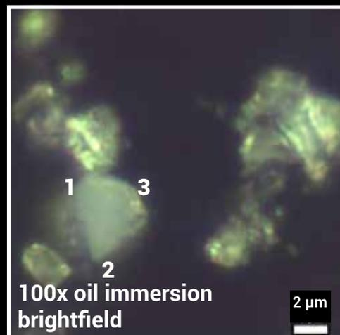
Above is the same area of the geological sample imaged with SMAL (on the left) and 100 x oil immersion in brightfield mode (on the right). The improved resolution allows SMAL to resolve the edge of the deposit (1,2,3) where it is blurred with conventional optical microscopy.
