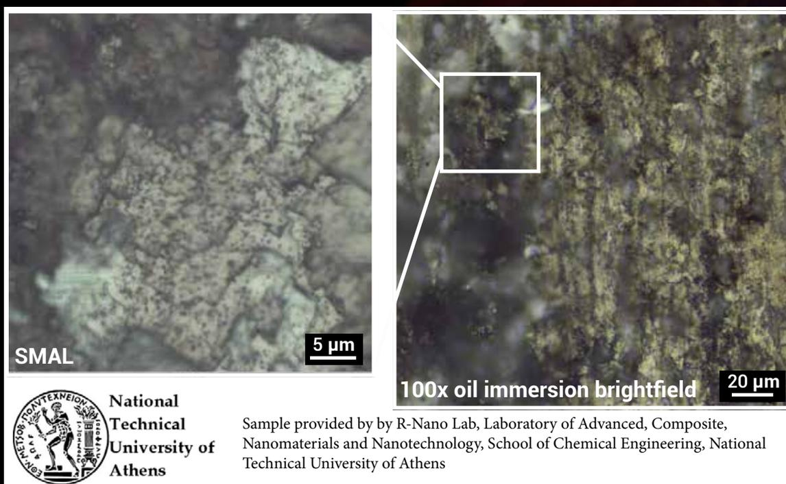
Above, the corroded metal is visible in the 100x image however the details of the oxidation are not resolved. In the SMAL image you can see the increased magnification and resolution reveal more details around the layers and points of corrosion. (Square added for scale reference and represents a similar area on the sample.)
