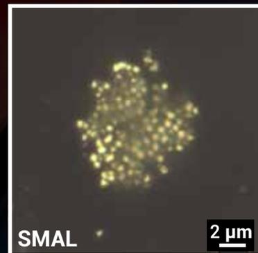
Above is a 20 x20  $\mu\text{m}$  image of a geological deposit taken with a 100x oil immersion lens. With standard optical microscopy you cannot make out the details of the specific deposits. In the SMAL images you can see the greater level of detail that SMAL yields. (Square added for scale reference and does not represent the same location on the sample.)
