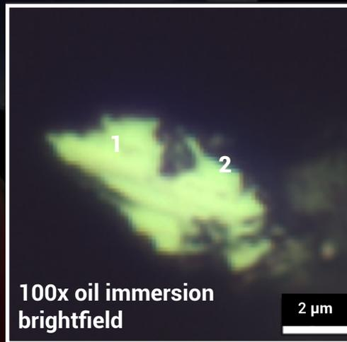
Above is the same area of the geological sample imaged with SMAL (on the left) and 100 x oil immersion in brightfield mode (on the right). The improved resolution of SMAL allows you to see the features on the face of the sample (1,2) which are undetected by conventional optical microscopy.
