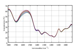
Infrared absorption spectra of a commonly used marine engine oil. The visible changes in the mid-infrared absorption spectra are directly related to the water absorption of the oil. A chemometric analysis of the spectra can be carried out using the Sphinx Suite software.
