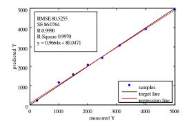
The results above are the results of a PLS1 analysis of the measured absorption spectra of the marine engine oils. The results are compared to the results of a reference analysis from a certified oil laboratory. The correlation between laboratory results and measured results are excellent.
