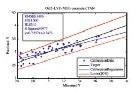
The Total Acid Number (TAN) has been calculated from the measured absorption spectra using the SphinxSuite software module. The plot compares the TAN obtained from analysing the mid-infrared absorption spectra to the TAN obtained from the same oil sample in an accredited oil analysis laboratory. The correlation between the results is exceptional.
