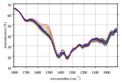
Mid-infrared absorption spectra of a typical marine engine oil at different points during the lifetime of the oil. Note the visible changes in the spectra which are related to specific oil degradation effects.
