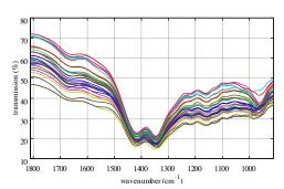
Infrared absorption spectrum of marine engine oils with different levels of soot contamination. The increased soot contamination is reflected as a baseline shift in the mid-infrared absorption spectra of the samples.
