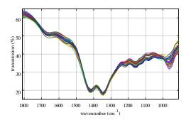
The results shown in the figure above are the baseline corrected mid-infrared absorption spectra of the marine engine oils. The baseline correction has been carried out using the SphinxSuite software module. Using the baseline correction the soot level contamination of an oil sample can be quantified.
