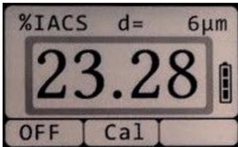
A high resolution display ensures clear visibility of conductivity values while still displaying additional information about the measurement. Calibration uses a "one point" calibration method to facilitate use. Certifiable standards are supplied with the unit.
