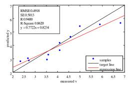
The i-pH value has been calculated from the measured absorption spectra using the SphinxSuite software module. The plot compares the i-pH values obtained from analysing the mid-infrared absorption spectra to the i-pH values obtained from the same oil samples in an accredited oil analysis laboratory. The data indicate that the oil reference data obtained from the oil laboratory should be checked as they indicate a saturation effect (systematic error of titration technique for i-pH value).
