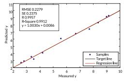
The Total Base Number (TBN) has been calculated from the measured absorption spectra using the SphinxSuite software module. The plot compares the TBN obtained from analysing the mid-infrared absorption spectra to the TBN obtained from the same oil sample in an accredited oil analysis laboratory. The correlation between the results is exceptional.
