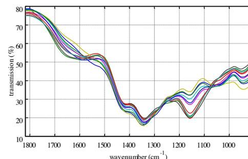
Mid-infrared absorption spectra of a typical biogas engine oil at different points during the lifetime of the oil. Note the visible changes in the spectra which are related to specific oil degradation effects.
