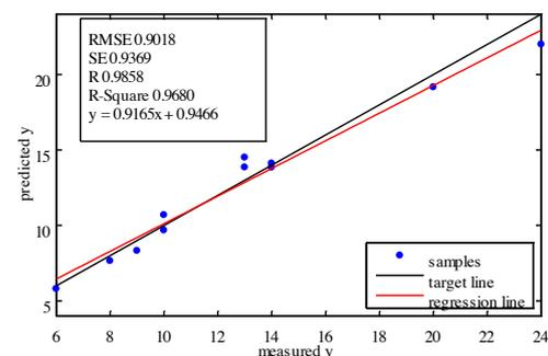
The oil oxidation has been calculated from the measured absorption spectra using the SphinxSuite software module. The plot compares the oil oxidation levels obtained from analysing the mid-infrared absorption spectra to the oxidation levels obtained of the same oil sample in accredited oil analysis laboratory. The correlation between the results is exceptional.
